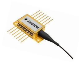
The 830nm series laser diodes are fabricated in a hermetically sealed 14-pin butterfly package. The laser diodes contain a monitor photodiode, thermoelectric cooler (TEC), and a thermistor to secure high-quality laser performance. Our laser products are Telcordia GR-468 qualified and in compliance with RoHS Directives.
